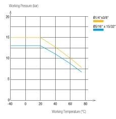
To calculate burst pressure, the values in this graph
